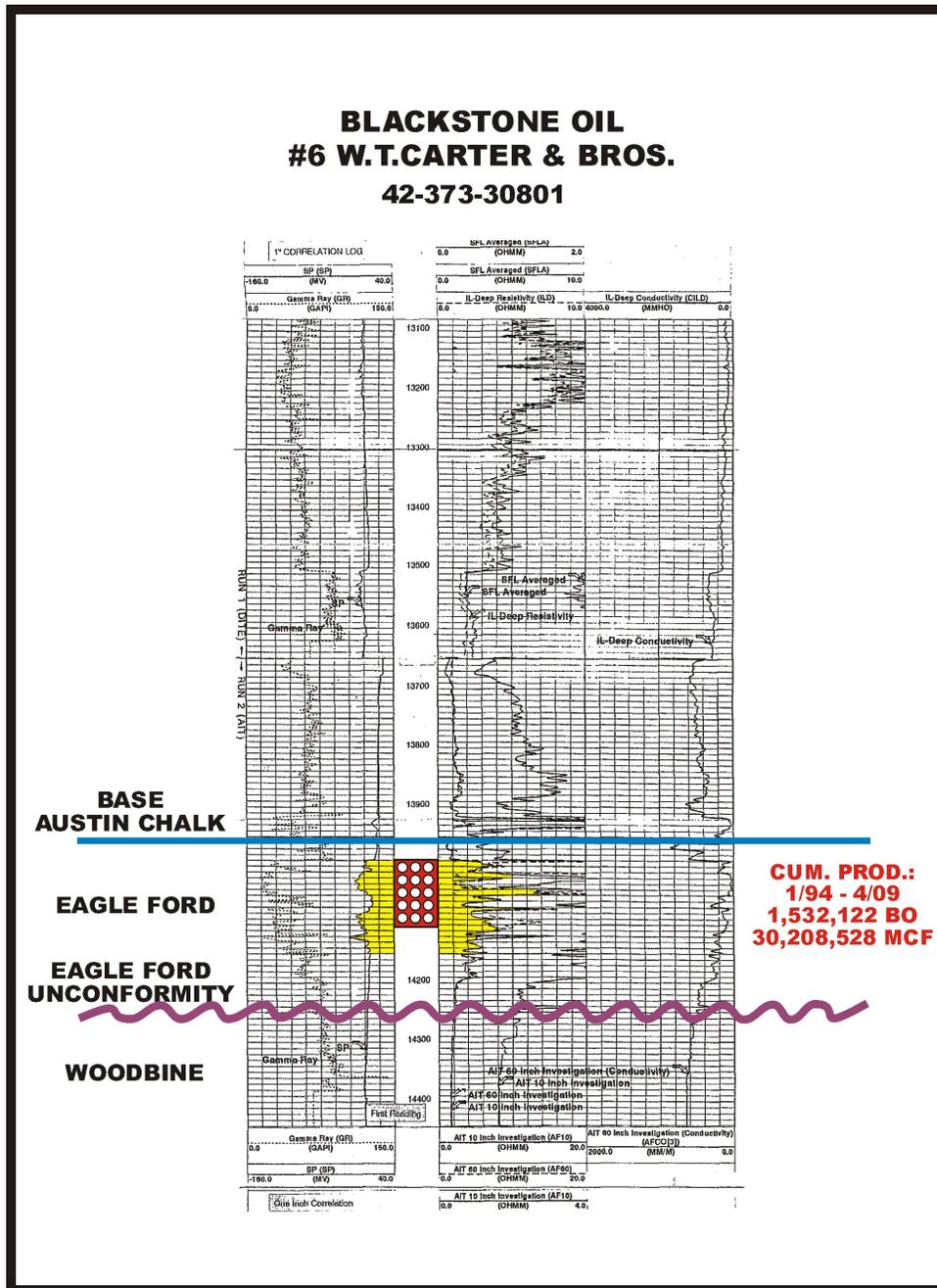
Figure 13. Log of the Blackstone #6 Carter well (API 42-373-30801), Double A Wells Field, Polk County, Texas. This well produces gas from Eagleford-aged sands within the Double A Wells incised valley.
