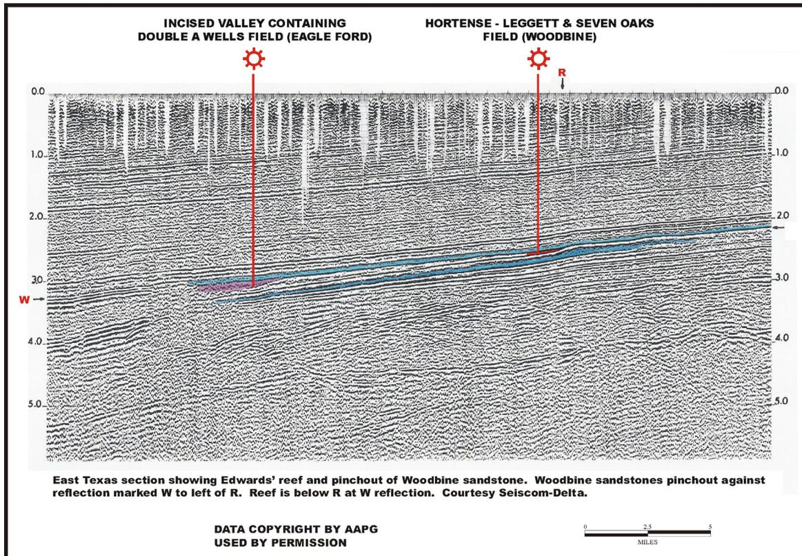
**Figure 12.** Published north-south seismic line showing the Edwards reef trend and the pinchout of the Woodbine, Polk County, Texas (modified after Sheriff, 1976). Purple wedge shows location of Eagle Ford incised valley at Double A Wells Field. This seismic line is parallel to log cross-section in [Figure 6C](#).
