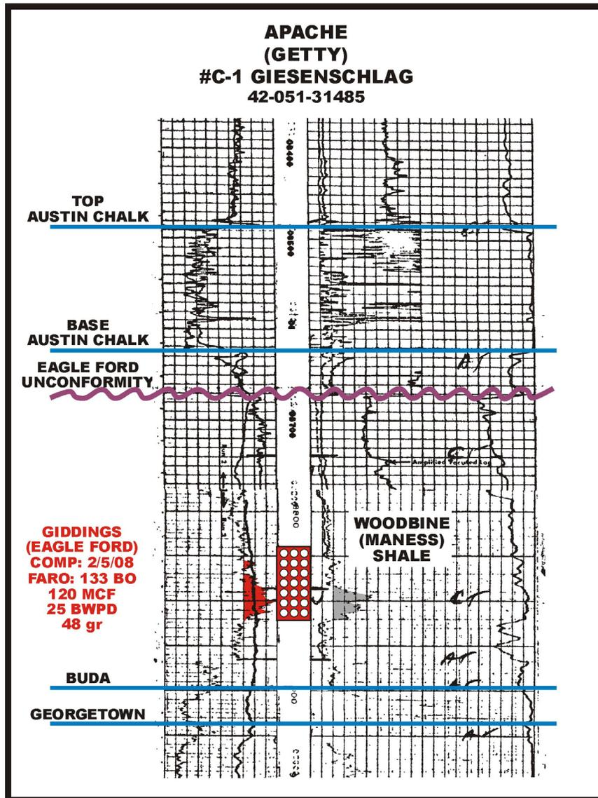
**Figure 7.** Well log of the Apache (formerly Getty) #C-1 Giesenschlag well (API 42-051-31485), Burleson County, Texas. This well produces oil from the lower Woodbine Maness Shale.
