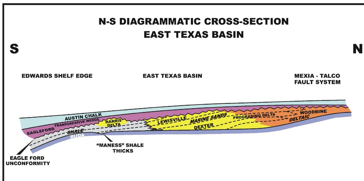
Figure 14. A north-south diagrammatic cross-section across the East Texas Basin which demonstrates the regional stratigraphy within the basin. Compare this to Figure 4 stratigraphy.
