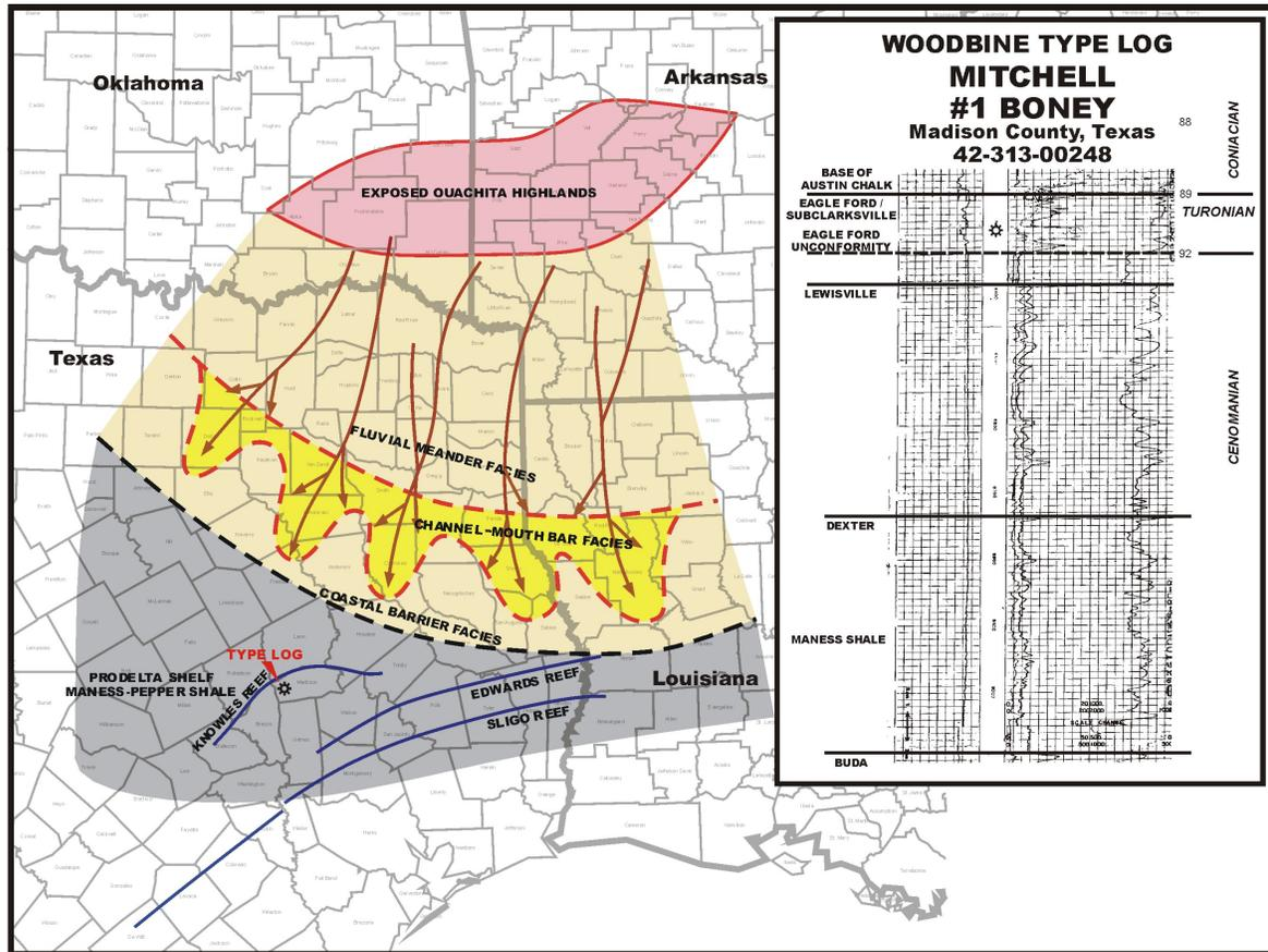
Figure 5. Paleogeographic map of the Lower Woodbine Dexter fluvial system interval (modified after Oliver, 1971).
